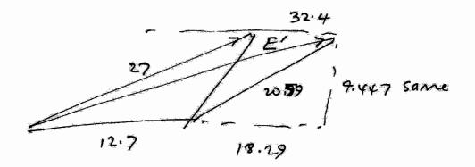
Increase  $E_{ph}$  by 20% from 27 kV to 32.40 kV.
