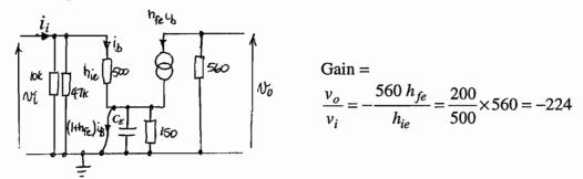
(e) With  $C_E$  omitted, the emitter-ground short is removed, with the capacitor itself. A current  $(1 + h_{fe})$  i<sub>b</sub> now flows thru emitter resistor  $R_E$ . Hence using KVL at the input:
