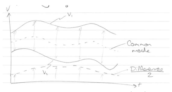
The common mode signal is the average of the two signals – i.e.  $\left(\frac{v_1 + v_2}{2}\right)$ . Normally
