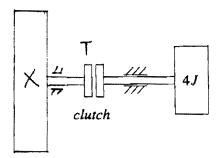
There must be an equivalent votating system consisting of a smale flywhul of unknown inertia, say X, fixed to a snaft which is colinear with the imput shaft and which is dunamically indistinguishable from the repectived system.
