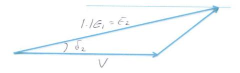
As the power is constant, and it is proportional to the perpendicular height of the above triangle, the load angle must decrease. The perpendicular height is  $E\sin\delta$ . =>  $E_1\sin\delta_1 = E_2\sin\delta_2$ .
