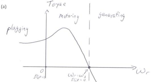
At synchronous speed, there is no relative motion between the stator field and the rotor, so the magnetic flux threading the rotor does not change => no rate of change of flux => no emfs induced in the rotor => no current flowing in rotor => no rotor magnetic field => no torque.
