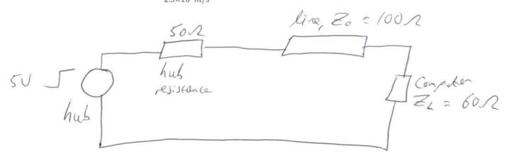
The first voltage pulse has an amplitude of  $5Vx \frac{100\Omega}{50\Omega + 100\Omega} = 3\frac{1}{3}V$
