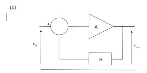
From the figure,  $V_{\text{out}} = A(V_{\text{in}} - BV_{\text{out}})$
