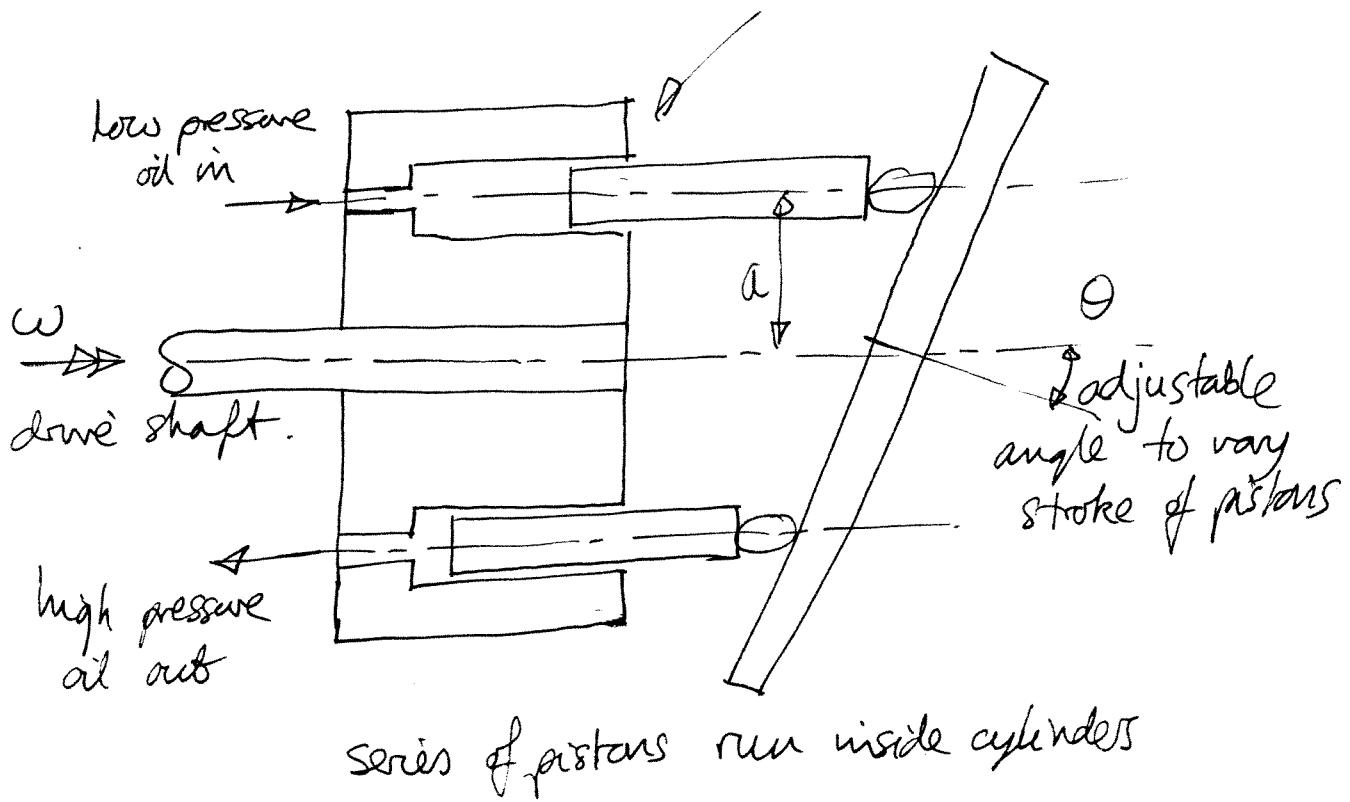
Inlet and outlet ports receive low pressure oil at top of stroke and generate high pressure at bottom of stroke.
