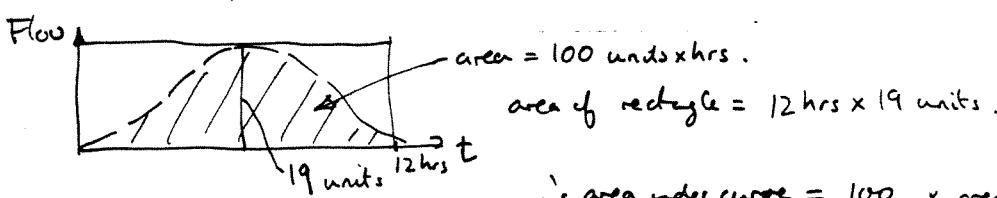
$$\therefore \text{area under curve} = \frac{100}{12 \times 19} \times \text{area of rectangle}$$
