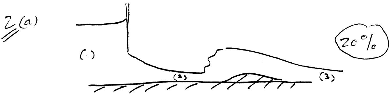
$$\text{Bernoulli} \quad S + \frac{v_1^2}{2g} = 1 + \frac{v_2^2}{2g}$$
