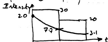
$\therefore$  Infiltration curve always under rainfall curve.
