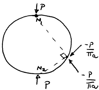
Superposition of forces at  $N_1$  &  $N_2$  gives hydrostatic pressure on a circle of radius  $a$ . Remove it by applying a hydrostatic tension
