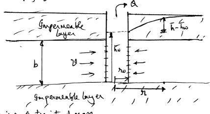
Empermeable layer, h, h, howing continuity of man  $Q = A \cdot D = 2\pi h b K \frac{dh}{dh}$
