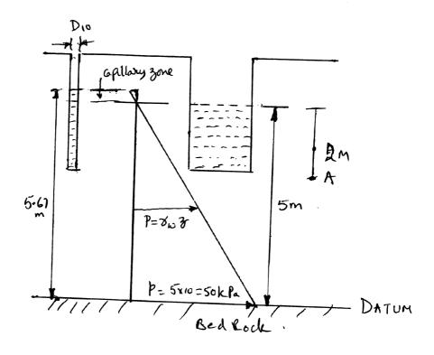
Potential head at point A 2m below the water table.
