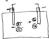
The Contaminents arriving at the electrodes are pumped out and removed. This method works well and contaminants are Contained preventing futher movement due to advection. Disadvantages are it is expensive and larg term.
