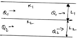
The hydraulic gradient driving the flow i' is the same for both layers.
