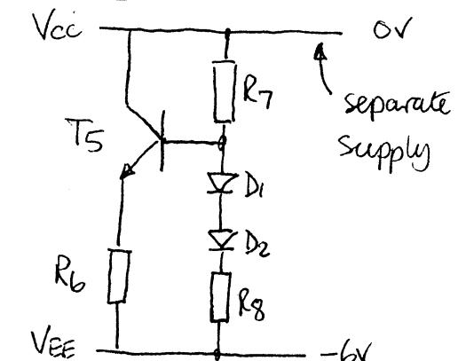
$R_7, R_8, D_1, D_2$  are a potential divider to set  $V_{BS}$  to  $(-1.5 + 0.8) V$
