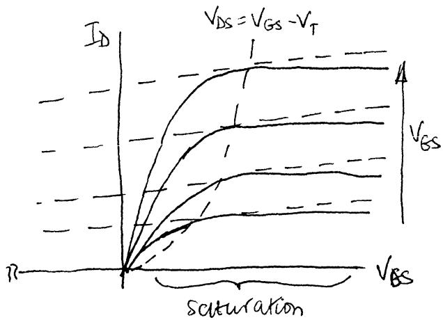
The near-constant current is a useful characteristic in linear circuits.
