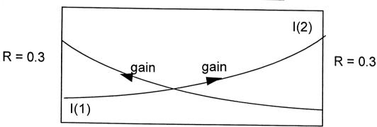
Assume that stimulated emission encounters a gain per unit length (due to stimulated amplification), G, and a loss per unit length due to scattering and absorption,  $\alpha$ , as it passes along the laser. The gain G in practice creates extra photons to compensate for those photons lost as the signal travels over a distance of unit length.
