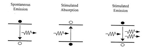
Spontaneous Emission: An electron in a high energy level falls losing energy which is emitted as a photon – the basis of operation of a light emitting diode.
