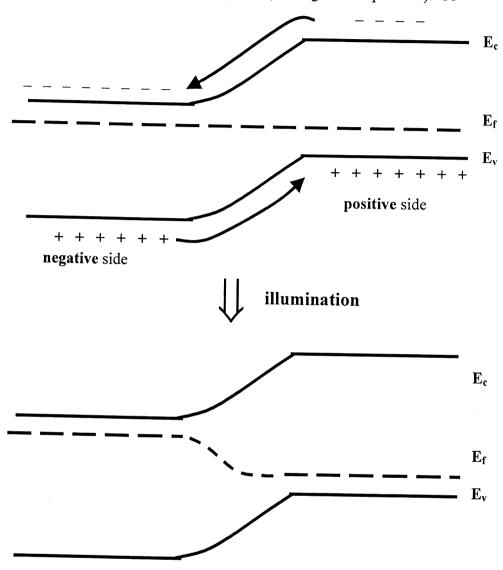
The bands become nearly flat  $\Rightarrow$  voltage (slightly less than bandgap voltage) is generated. So the solar cell can be considered as a current generator connected in parallel with a diode.
