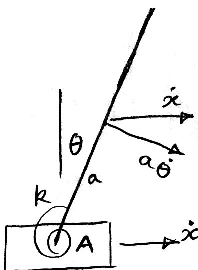
$$\begin{aligned} T &= \frac{1}{2}M\dot{x}^2 + \frac{1}{2}M(\dot{x} + a\dot{\theta}\cos\theta)^2 \\ &\quad (\text{trolley}) + \frac{1}{2}M(a\dot{\theta}\sin\theta)^2 \\ &\quad + \frac{1}{2}\left(\frac{1}{3}ma^2\right)\dot{\theta}^2 \\ &\quad (\text{rod}) \end{aligned}$$
