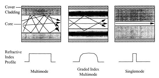
Single mode (SM) fibre is extensively used for long haul telecommunications. Almost all of the digital telephone networks in the UK uses silica based single mode optical fibre. Silica SM fibre has very low attenuation per unit length, especially at the two main comms wavelengths, 1310 and 1550nm.
