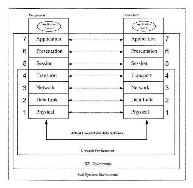
b) Layer 1: The physical layer. This defines an interface in terms of the connections, voltage levels and data transmission rate, in order for signals to be transmitted bit by bit. The function of the physical layer is to provide a 'virtual bit-pipe' service to the data link layer of the OSI reference model. At the lower interface of the physical layer, we have the physical communications channel. This may be using any of the physical media available for transmission of data.
