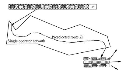
The individual packets will be routed as per their native protocol outside of the MPLS network, however across the MPLS network, the routing will be path oriented as this minimises delay at each node in the MPLS network. Routing in therefore path oriented.
