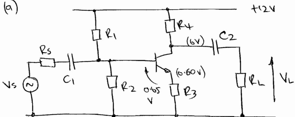
Bias resistors  $R_1, R_2$
