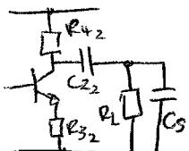
(c) We need to monitor the audio signal amplitude  $\therefore$  use a diode demodulator on the output of stage 1 and use this to control a MOSFET analogue switch to control the signal path to  $R_L$  (note we need stage 2 as a buffer or switching  $R_L$  will alter the output level being monitored)
