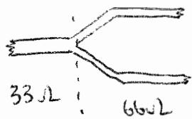
For matching  $Z_0 = 66\mu L$   $\therefore w = 0.92 \text{ mm}$
