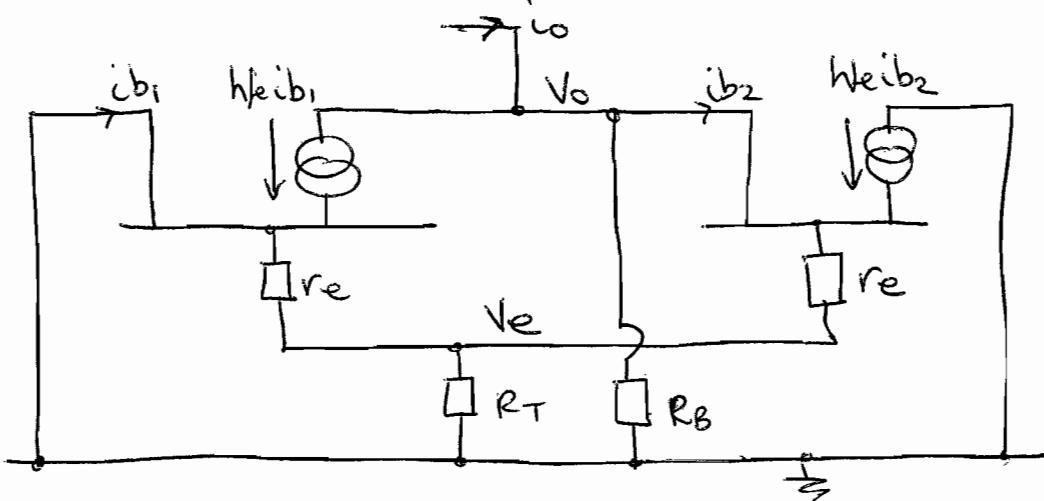
$$\textcircled{1} \quad V_e = h_{fe} (i_{b1} + i_{b2}) R_T, \quad V_e = -h_{fe} i_{b1} r_e \quad \textcircled{2}$$
