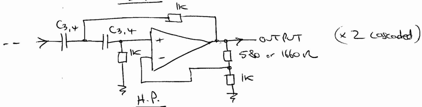
$$\text{For L.P. } f_c = \frac{1}{2\pi f_m R C_{1,2}} = 7 \times 10^6, \quad R = 1 \text{ k}\Omega \text{ throughout}$$
