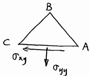
Because both AB and BC surfaces are stress free, hence  $\sigma_{yy} = \sigma_{xy} = 0$  on AC. Therefore, the whole extrusion is free of stress.
