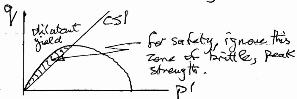
Impact : Failure of trenches & cuttings e.g. in London Clay.
