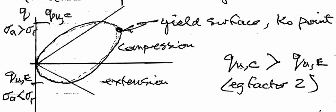
Impact: dangerous just to do compression tests on vertical cores if there are "passive" zones — as with foundations of embankments,
