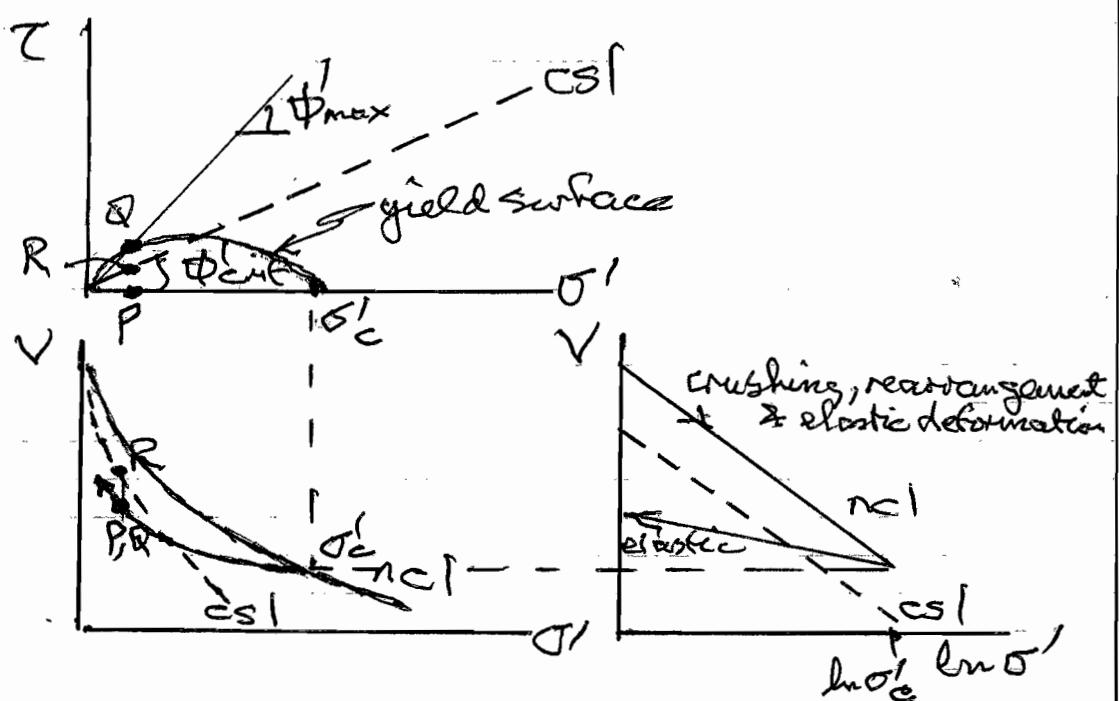
When sheared from high overconsolidation ratio ( $\sigma'_c / \sigma'$ ) at P, "drained" peak strength at Q falls to critical state strength at R as the soil dilates. So "friction angle"  $\phi_{\max} \approx \phi_{ult} + \psi$  where  $\psi$  is the angle of dilation (which varies).
