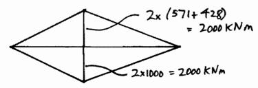
(b) Note that the beam specified in (b) is the mirror image of the beam in (a), and also that the stiffness is now twice the stiffness in (a).
