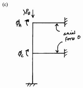
Key difference from case (b) is that member AC has non-zero rotations at both ends.
