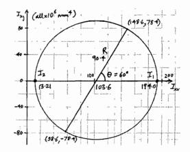
Nearest section is  $356 \times 171 \times 67$  Universal Beam ( $I_{xx} = 19640 \text{ cm}^4$ ;  $I_{yy} = 1362 \text{ cm}^4$ ), but area is  $85.5 \text{ cm}^2$  whereas our section has  $76.40 \text{ cm}^2$  (so  $9.1 \text{ cm}^2$  missing).
