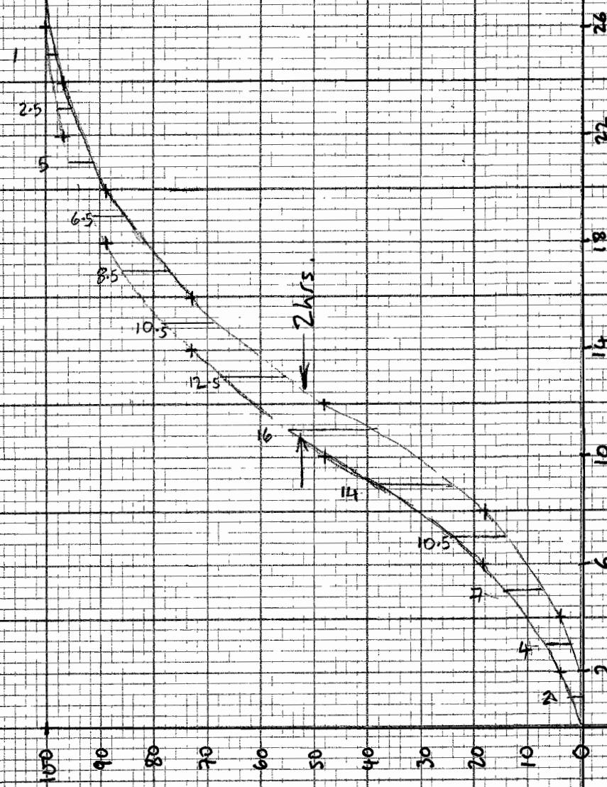
$$Q2 \quad a) \quad \text{Energy} \quad E = d + \frac{V^2}{2g} = d + \frac{Q^2}{2gA^2}$$
