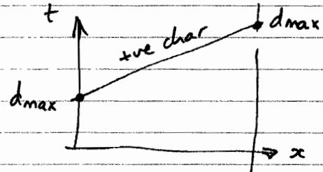
$$\begin{aligned} \text{Now } d(x=0) &= 3 + \Delta h \text{ metres} \\ &= 3 + 2(1 - \cos(\pi t/8)) \\ &\quad \cos \frac{2\pi t}{16} \end{aligned}$$
