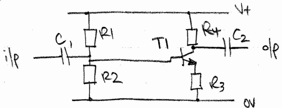
$R_1, R_2$  base bias resistors : define input impedance and aim to set  $V_c \approx V_{apply}/2$
