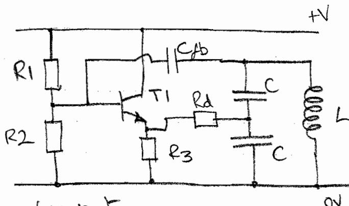
$T_1$  : transistor $R_1 + R_2$  : base bias resistors $R_3$  : emitter load resistor $L + C$  : resonant circuit $C_{fb}$  : feedback capacitor $R_d$  : drive resistor
