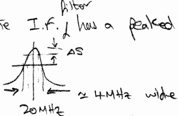
Frequency is modulated around 20MHz (I.F.), so the amplitude will drop each side - hence the FM signal will be mixed into the AM signal.
