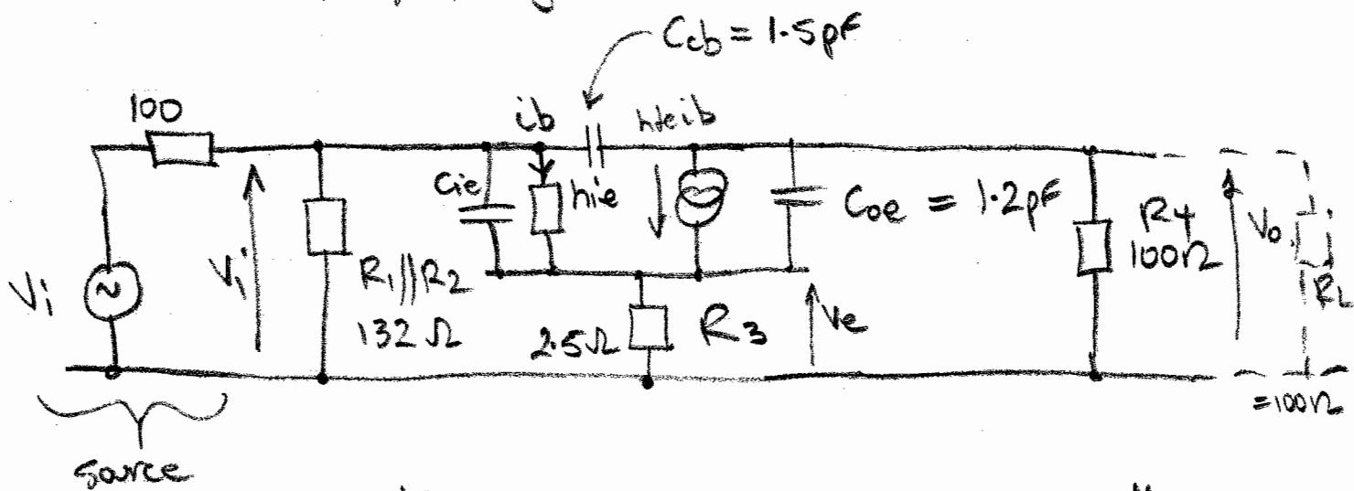
Net amplifier gain  $\frac{V_o}{V_i} = -20 \quad \therefore$  Miller effect on
