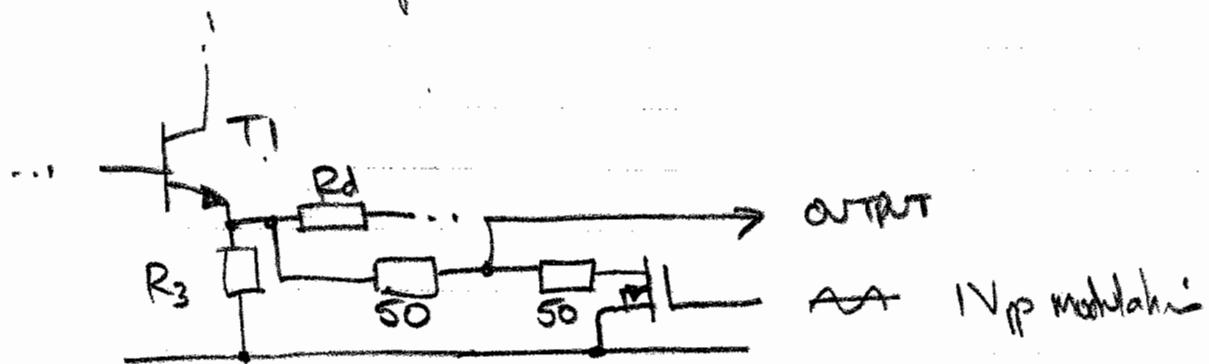
(or, more elegantly, the main oscillator transistor base bias could be modulated through  $\sim 1k\Omega$  resistor).
