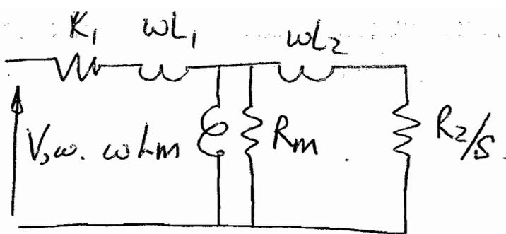
When commissioned as part of a variable speed drive,  $V/f = \text{const}$ , so  $\frac{V}{\omega L_m}$  and smallish. Since  $\omega$  is variable, the value of  $R_2/s$  should be large compared to  $R_1$  and  $\omega L_1$ , under all conditions (i.e. we work at small  $s, \omega$ ).
