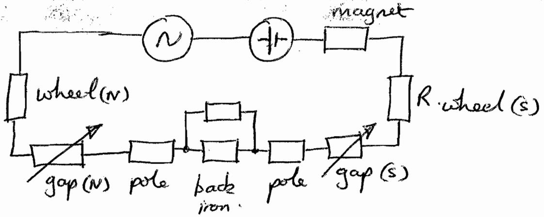
The torque maybe calculated using reluctance & energy stored in the gap.
