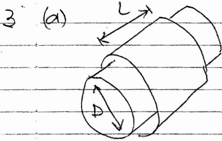
In a 'long' bearing axial flow of lubricant is negligible, which means that axial pressure gradients are small w.r.t those around circumferential.
