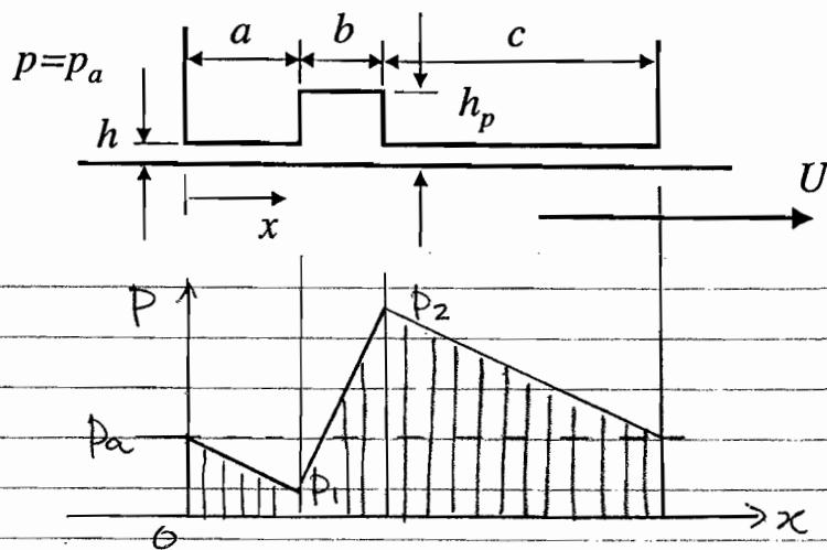
possible for shaded area  $> p_a(a+b+c)$  so some load carrying capacity.
