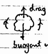
At terminal velocity, no acceleration, so no net force
