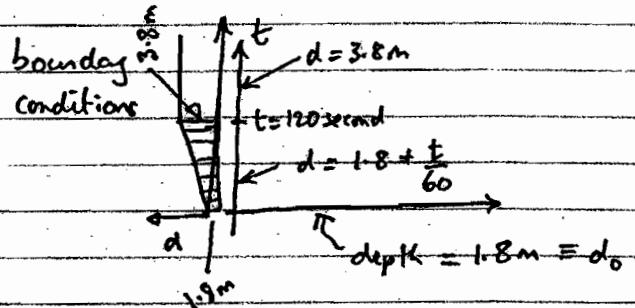
From data sheet:  $u - 2c = k_1$ , const on any -ve characteristic
