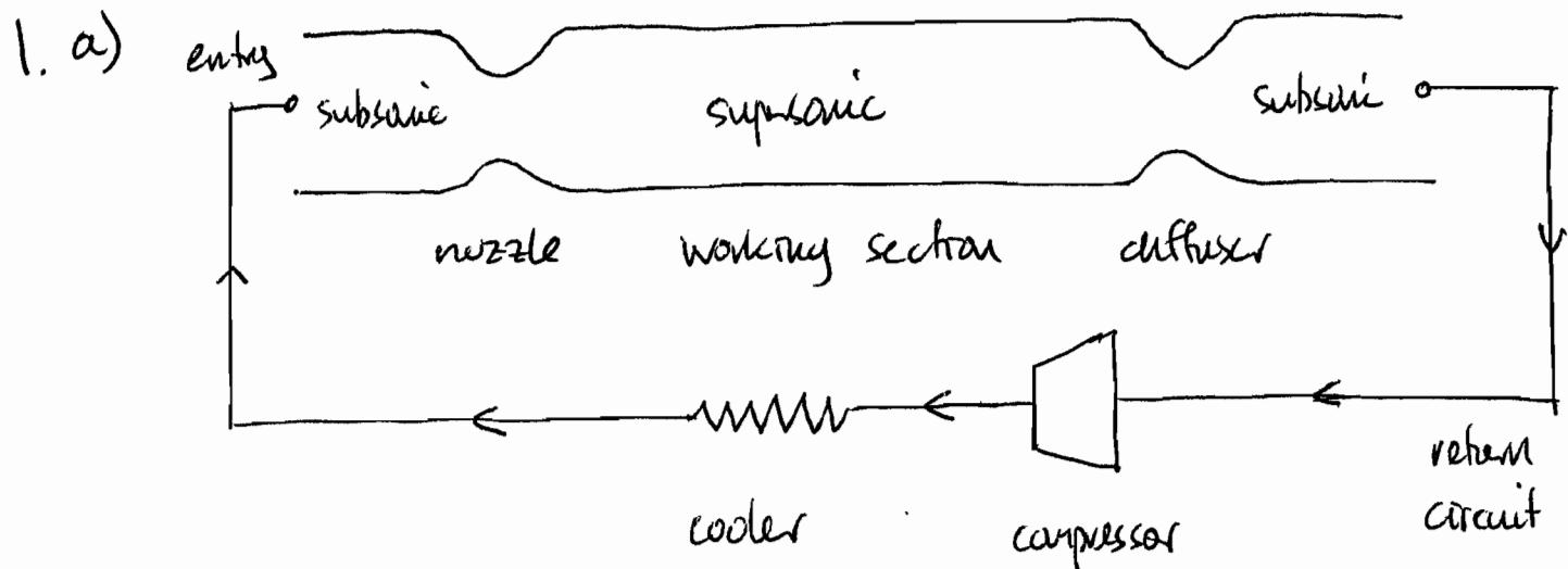
The tunnel must accelerate the flow from subsonic through  $M=1.0$  at the nozzle throat up to  $M=3.0$  on the working section. It must then decelerate the flow back to subsonic after the diffuser throat. The compressor restores the stagnation pressure back to the value at entry while the cooler restores the stagnation temperature downstream of the compressor back to the value at entry.
