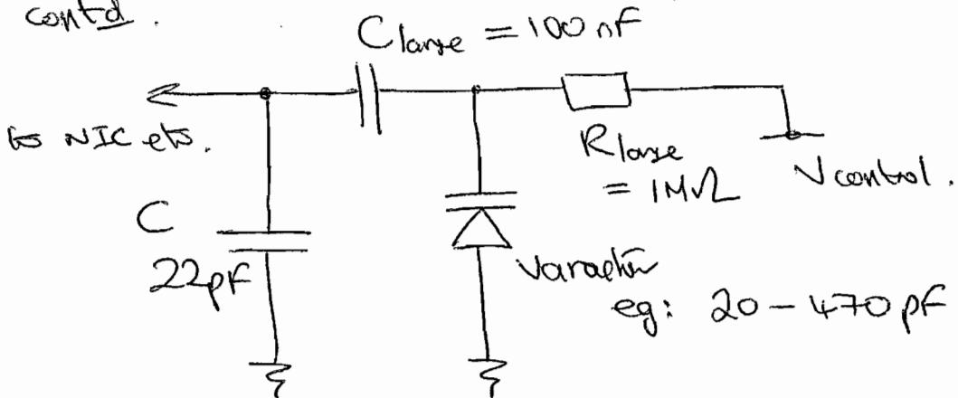
Let's assume the varactor can vary  $20 - 470\text{ pF}$ , hence with  $C = 22\text{ pF}$ , the total capacitance varies  $42 - 492\text{ pF}$  (i.e. just over 10:1 range).
