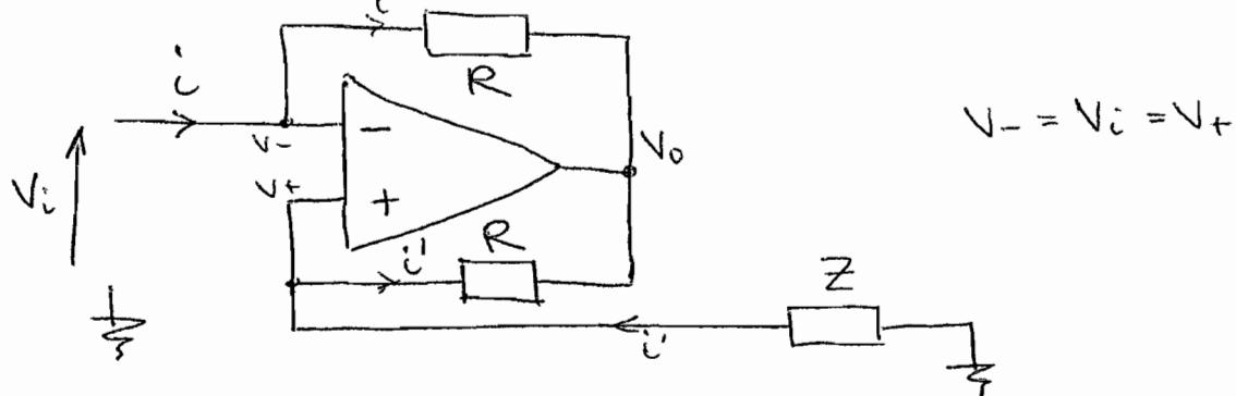
As  $V_+ = V_-$  then the voltage across the impedance  $Z = V_i$  and since  $(V_o - V_i)$  appears across both + and - feedback resistors then  $i' = i \Rightarrow V_+ = -iZ \therefore V_i = -iZ$ , hence the input impedance  $\frac{V_i}{i} = -Z$ .
