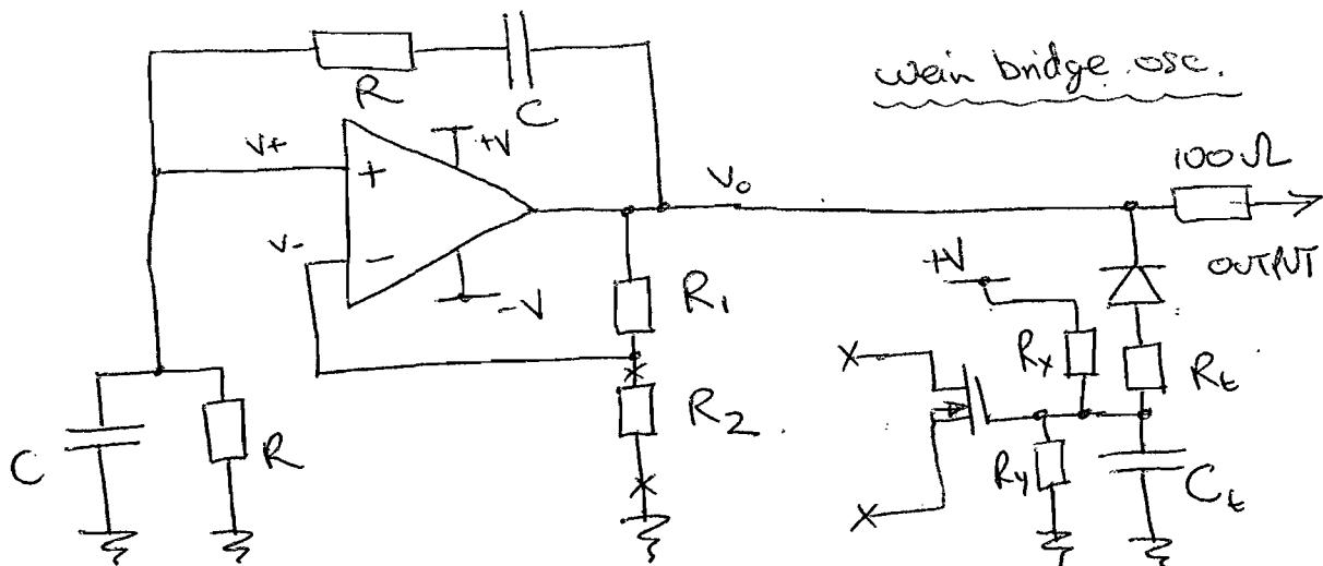
$$V_+ = V_o \cdot \frac{\frac{R}{1+j\omega CR}}{\frac{R}{1+j\omega CR} + R + \frac{1}{j\omega C}} = \frac{1}{1 + \frac{R + \frac{1}{j\omega C}}{\frac{R}{1+j\omega CR}}}$$
