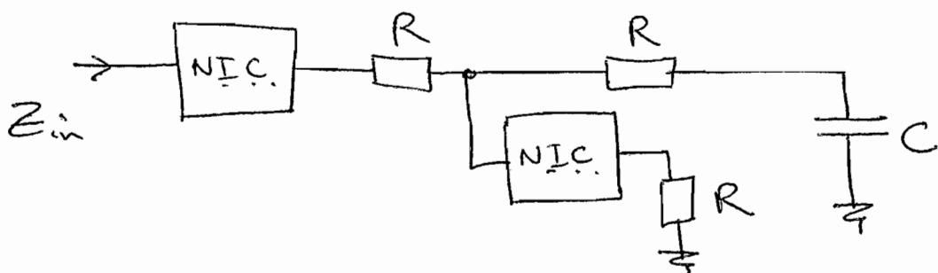
$$\begin{aligned} Z_{in} &= - \left[ R + -R \parallel \left( R + \frac{1}{j\omega C} \right) \right] \\ &= - \left[ R + \frac{-R \left( R + \frac{1}{j\omega C} \right)}{-R + R + \frac{1}{j\omega C}} \right] \\ &= - \left[ R - \frac{R^2 j\omega C - R}{R^2 j\omega C} \right] = j\omega C R^2 = j\omega L \end{aligned}$$
