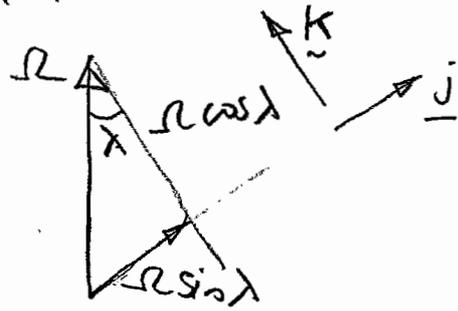
Next resolve the  $\Omega \cos \lambda$  component into its  $\underline{i}$  &  $\underline{k}$  components
