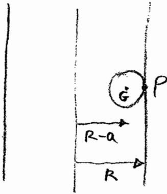
(a) P in the ball is at rest (no slip) and G is moving on a horizontal circle
