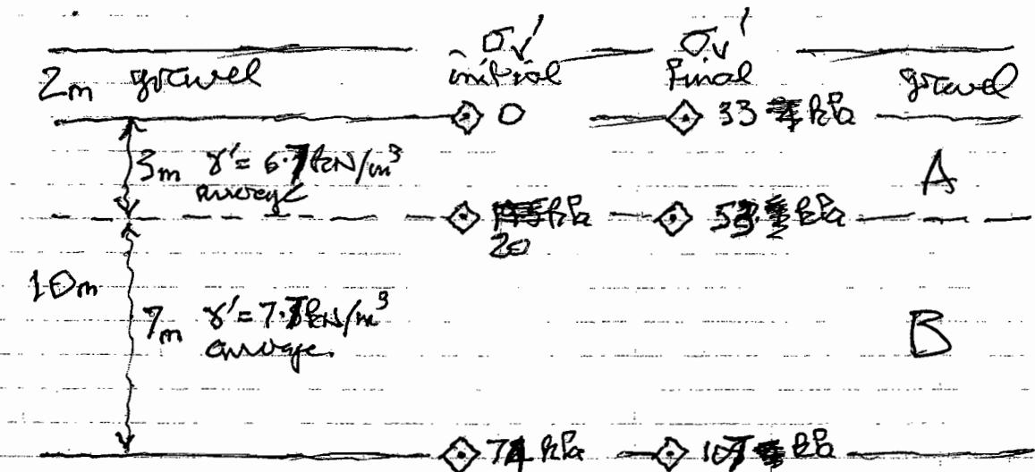
In (b) we calculated  $\gamma = 16.5 \text{ kN/m}^3$  for clay at 50kPa. An iteration shows that  $\sigma'_v \text{ initial} \approx 20 \text{ kPa}$  at 3m depth in the clay, so this is chosen as layer A with an average unit weight of  $16.5 \text{ kN/m}^3$  so that  $\gamma' = 6.7 \text{ kN/m}^3$ .
