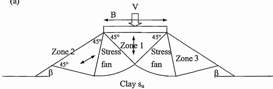
The stress fan has an angle of  $90^\circ - \beta$ .
