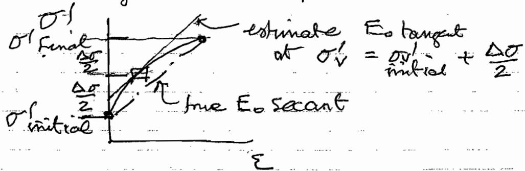
For the top layer A, using  $E_0 = \frac{\sigma'_0 V}{z}$
