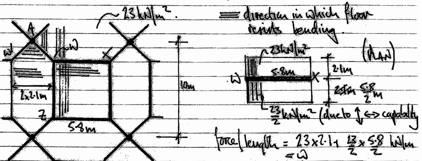
$$\text{force/length} = 23 \times 7.1, \frac{23}{2} \times \frac{5.8}{2} \text{ kN/m}$$
