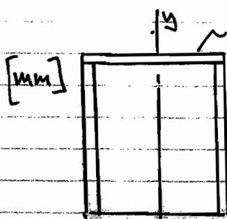
$$I_{yy} = 2 \times \left[ \frac{25 \times 450^3}{12} + (1150 \times 7.5) \times \left[ \frac{450 - 7.5}{2} \right]^2 \right] \text{ mm}^4$$
