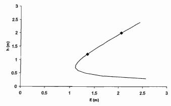
The critical depth for  $q = 2 \text{ m}^2/\text{s}$  is  $h_c = \left(\frac{2}{\sqrt{g}}\right)^{2/3} = 0.74 \text{ m}$  and  $E_c = 1.5 h_c = 1.11 \text{ m}$ , so road height should be  $E_1 - E_c = 0.941 \text{ m}$
