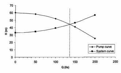
(d) When the pump runs at 1200 rpm, suppose it generates a discharge  $Q_{p2}$  against head  $H_{p2}$  with the corresponding operation point at the speed of 1000 rpm being  $Q_{p1}$  and  $H_{p1}$ . Then,
