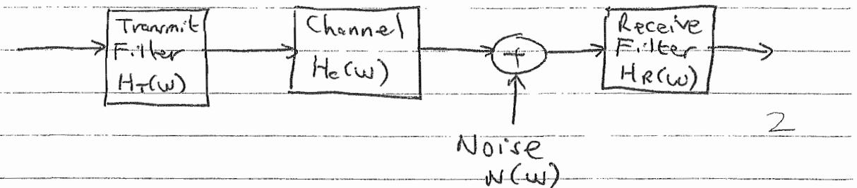
$H_T(w)$  shapes transmitted power spectrum. 1 $H_c(w)$  is the channel frequency response 1 $H_R(w)$  reduces the effect of noise. 1 $N(w)$  is the additive noise power spectrum
