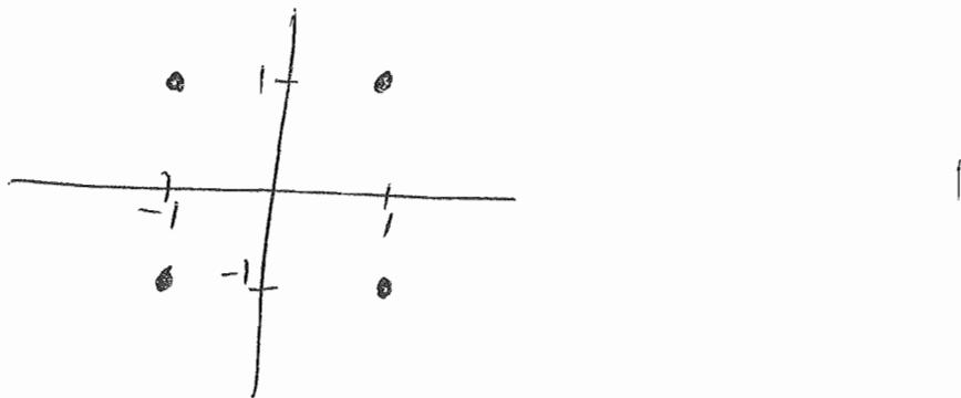
and conveys only 2 bits per symbol, compared with 6 bits per symbol for 64-PSK & 64-QAM.
