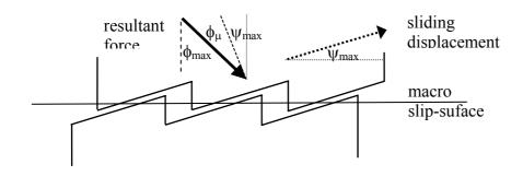
Intergranular angle of friction at sliding contacts  $\phi_{\mu}$
