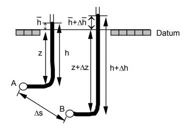
Total gauge pore water pressure at A:  $u = \gamma_w h = \gamma_w (\overline{h} + z)$
