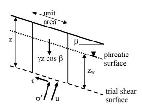
$$\begin{array}{ll} u &= \gamma_w z_w \cos^2\!\beta \\ \sigma &= \gamma z \cos^2\!\beta \\ \sigma' &= (\gamma z - \gamma_w z_w) \cos^2\!\beta \\ \tau &= \gamma z \cos\!\beta \sin\!\beta \end{array}$$
