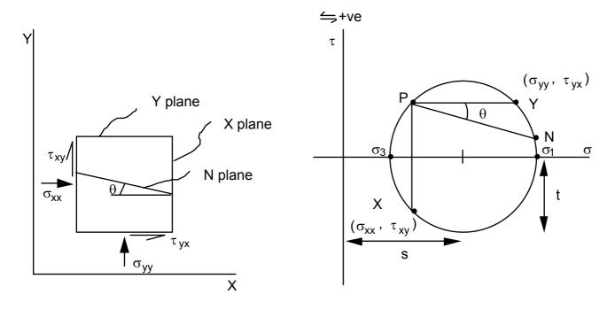
*Poles of planes P*: the components of stress on the N plane are given by the intersection N of the Mohr circle with the line PN through P parallel to the plane.
