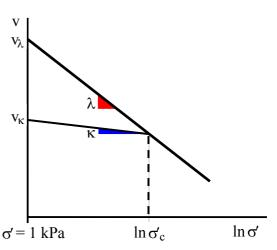
Plastic compression stress  $\sigma'_c$  is taken as the larger of the initial aggregate crushing stress and the historic maximum effective vertical stress. Clay muds are taken to begin with  $\sigma'_c \approx 1$  kPa.
