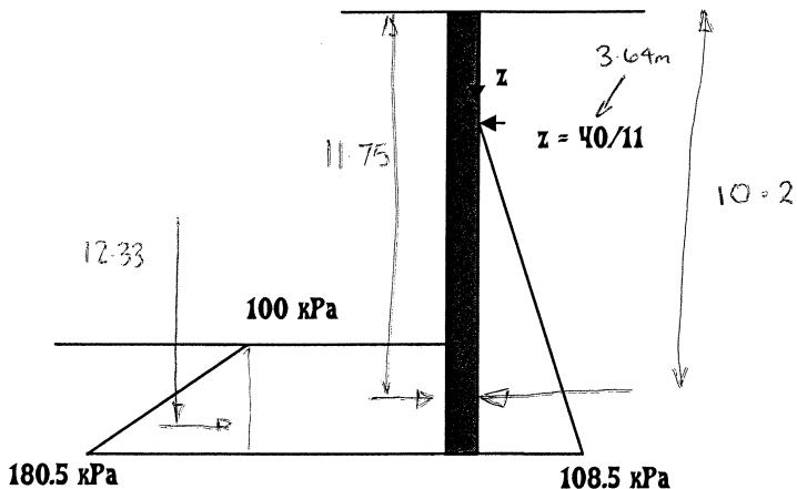
It is assumed that dry crack is formed at the location of negative pressure on the active side. Hence, the active pressure is zero down to  $z = 40/11 = 3.64$  m.
