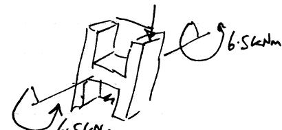
$$G = \frac{E}{2(1+\nu)} = \frac{30 \times 10^9 \text{ N m}^{-2}}{2(1.2)} \\ = \underline{\underline{12.5 \times 10^9 \text{ N m}^{-2}}}$$
