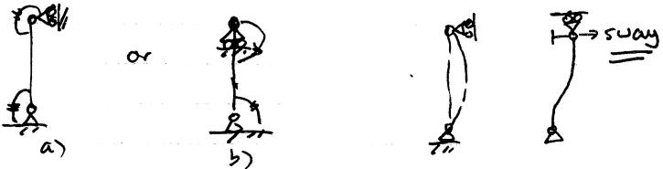
Construction details that might provide sway bracing include shear walls, cross-braced bays or stiff shear walls around say lift shafts + service cores.
