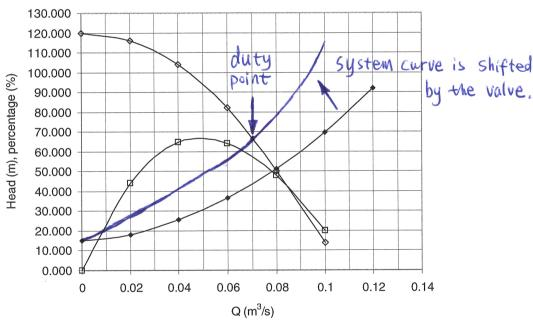
The system will curve will shift upwards to intersect with the pump curve at
