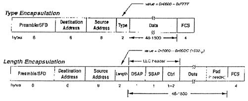
After removing the collision mechanism we are basically left with a transport frame format.
