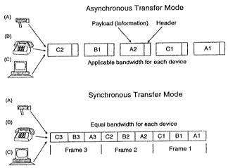
One possible solution is B-ISDN called asynchronous transfer mode or ATM.
