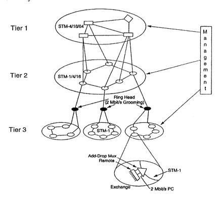
One solution is to replace the local exchanges with small remote concentrators (mux units) and connect these to the main exchanges with synchronous links. Local exchanges in tier 1 are replaced with an add/drop mux and remote concentrators working up to the STM-1 level. The mux units are used to form a basic ring structure.
