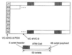
The advantage of the STM-1 frame is that it offers a huge wealth of virtual bandwidth as well as management services which will make ATM or IP over SDH easier than just pure ATM or IP systems. In ATM, the cell is limited to 53bytes, a 48 byte payload and a 5 byte header. ATM is defined at a transmission rate of 155.52Mbits/sec to be compliant with SDH and SONET.
