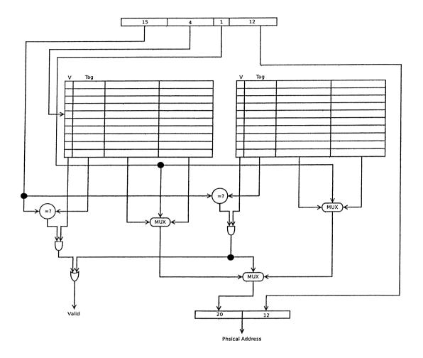
(d) Assume a MUX or testing equality takes two gate delays and that a table lookup takes six gate delays. If each gate causes a delay of 0.5ns, how long does your design of TLB take to compute a physical address?
