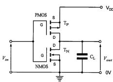
Note that since both devices have the sam e k and  $|V_T|$ , delays and r ise/fall times are the same for both transitions, 0-1 and 1-0.
