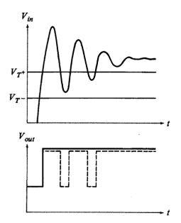
The output of a si mple inverter with switch level  $V_{\rm ID}$  would exhibit addition al spurious pulses.
