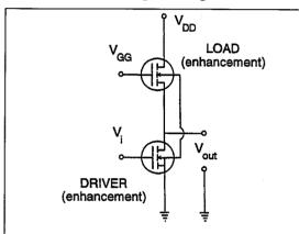
In circuits where resistive loads are unavoidable (for example, pseudo-nMOS logic or linear circuits), an appropriately biased MOSFET may be used as load, with the gate returned to a fixed bias to obtain an appropriate channel conductance, approximating the behaviour of a resistor. Static and dynamic logic gate performance are now a sensitive function of the dimensions of load and driver FET. Use of a depletion-mode FET with grounded gate is also possible.
