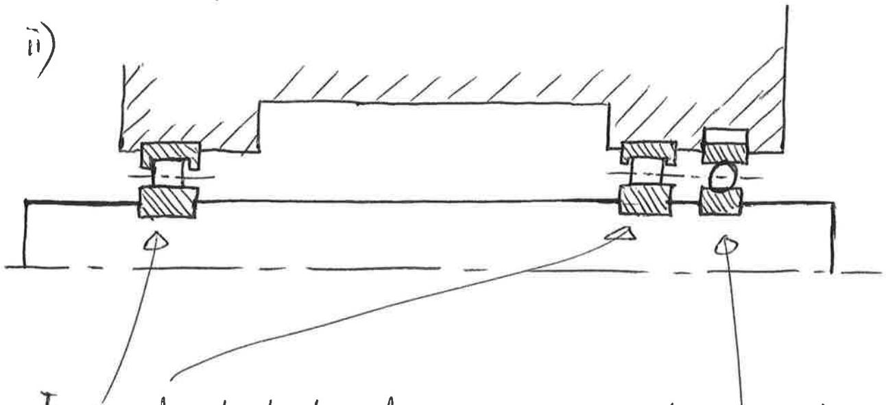
Inner and outer tracks of the roller bearings are positively located in radial and axial directions. Roller bearing cannot take axial load.
