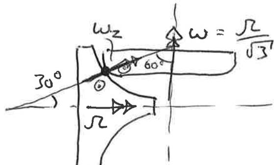
$$\begin{aligned} \omega_z &= \sqrt{2} \cos 30^\circ - \omega \cos 60^\circ \\ &= \sqrt{2} \frac{\sqrt{3}}{2} - \frac{\sqrt{2}}{\sqrt{3}} \cdot \frac{1}{2} \\ &= \frac{\sqrt{2}}{2} \left( \sqrt{3} - \frac{1}{\sqrt{3}} \right) = \frac{\sqrt{2}}{\sqrt{3}}. \end{aligned}$$
