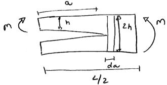
For its of specimen (one work typ):  $U = \frac{6m^2}{EB} \left[ \frac{L}{2} - a + a \right]$  when crack grows da
