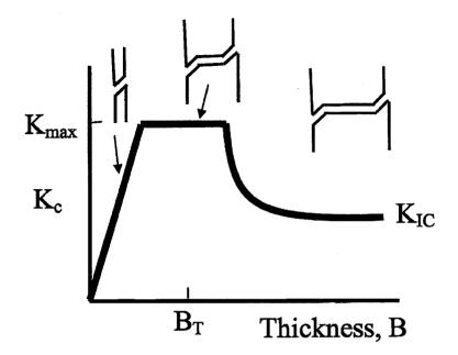
The plane strain asymptote of  $K_{\rm C}=K_{\rm IC}$  is attained when the thickness B attains the value  $B\geq 2.5(K_{IC}/\sigma_Y)^2$ . In thick specimens that exceed this criterion, shear lips form at the edges of the specimen of width about equal to  $r_p=\frac{1}{\pi}(K_{IC}/\sigma_Y)^2$ . There is high plastic constraint directly ahead of the crack tip such that the tensile stress =3  $\sigma_Y$ . This promotes both cleavage and microvoid coalescence.
