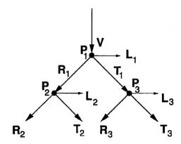
The tree is *constructed* top down, until either a ray fails to intersect an object or some predetermined maximum depth is reached. The tree is then *evaluated* bottom-up, as each node's intensity is computed from its children's intensities.
