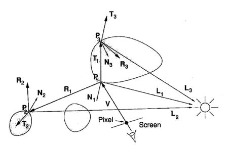
Simple ray tracing algorithms operate in world coordinates. A ray V is fired from the centre of projection through every pixel on the screen. When the ray strikes an object at  $P_1$ , further rays are spawned. One ray,  $L_1$ , heads for the *i*th light source. If  $L_1$  passes through other objects on the way, then the illumination intensity is attenuated by a shadow factor  $S_i$ , depending on the number and opacity of objects in the way.
