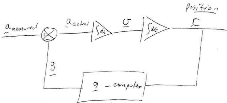
If integration is notoriously sensitive to drift and low-frequency instabilities so inertial navigation using accelerometers & rate gyros is only useful for short periods of time between recalibration events.
