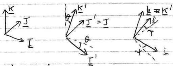
$$\begin{aligned} \underline{\omega} &= \dot{\theta} \underline{J} + \dot{\varphi} \underline{k} \\ \text{But } \underline{I}' &= \underline{I} = j \cos \varphi + i \sin \varphi \\ \therefore \underline{\omega} &= \dot{\theta} \sin \varphi \underline{i} + \dot{\theta} \cos \varphi \underline{j} + \dot{\varphi} \underline{k} \end{aligned}$$
