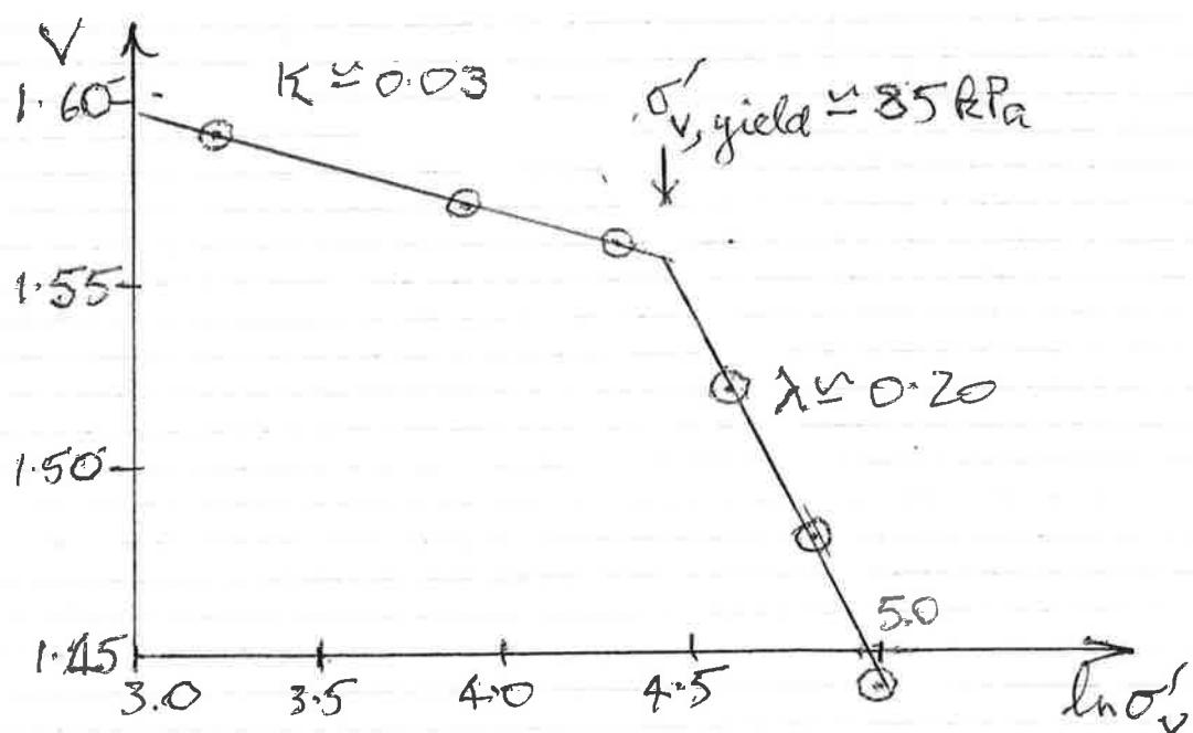
2(a) If we use the sample as representative, and take  $\sigma'_v$  from 25 kPa to 122 kPa, we get to  $\ln \sigma'_v = 4.80$ ,  $v = 1.49$ . So treating 10m of clay like an oedometer
