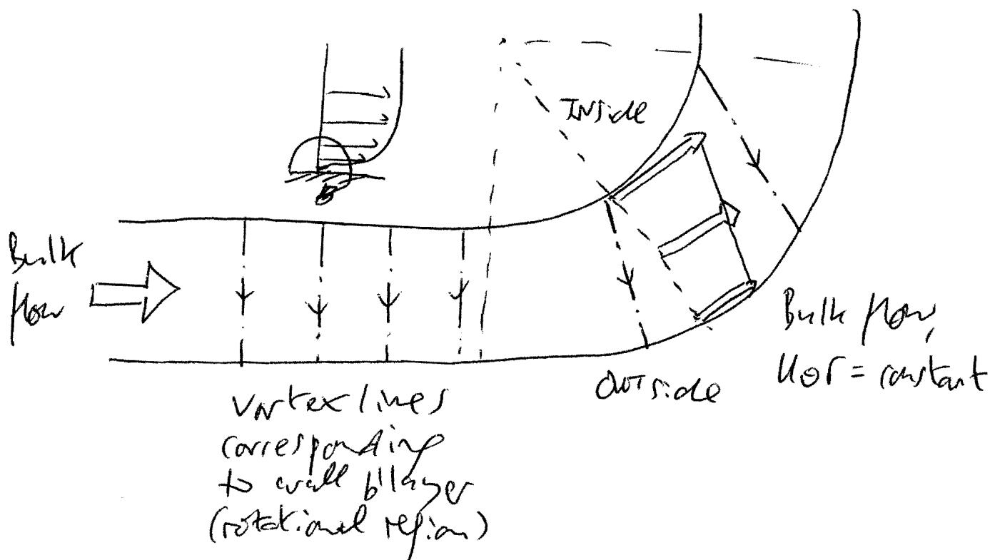
The bulk outer flow is slower than the inner ( $u_{\theta 1} = r_{\theta 1}$ ) hence vortex lines become increasingly rotated relative to radial lines ( $D\phi/Dt = 0$ ). Thus a streamwise component of vorticity - second =  $\omega_z$  flow - develops within the endwall b/layer
