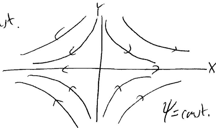
(iii) for inviscid flow the wall b/c  $\Rightarrow$  zero normal velocity so any stream line could be a wall — for our purposes,  $Y = 0$ .
