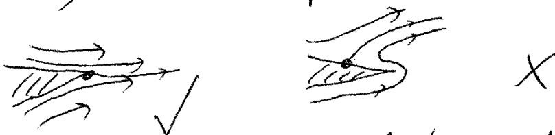
A range of irrotational flows about a flat plate can be derived by conformal mapping of irrotational flows of varying circulation about a cylinder. The Kutta condition allows us to select a physically meaningful value for the circulation.
