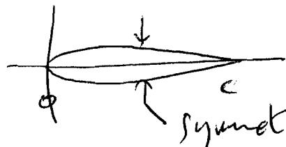
Streamlines:  $\frac{v'}{U} \Big|_{T=0^+} = \frac{1}{2} \frac{dt}{dx} ; \frac{v'}{U} \Big|_{T=0^-} = -\frac{1}{2} \frac{dt}{dx}$ .
