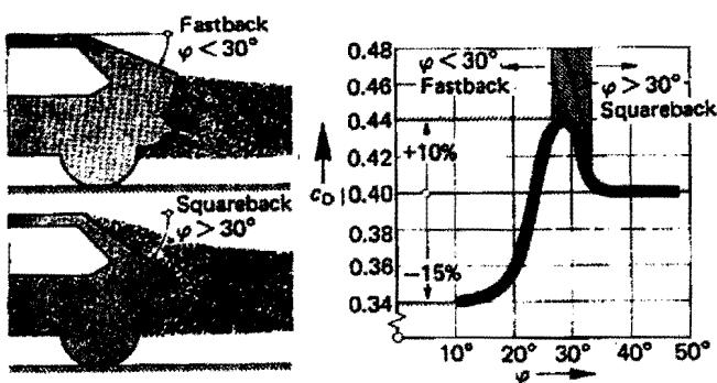
Typical angles for well-designed fastback shaped cars are around 20 degrees.
