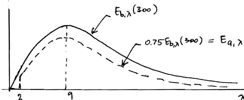
(iii) THE ABSORBER COATING IS TRANSPARENT TO THE SHORT WAVELENGTH OF SUNLIGHT, BUT OPAQUE TO THE LONGER WAVELENGTHS EMITTED BY THE ABSORBER, thus trapping radiative power.
