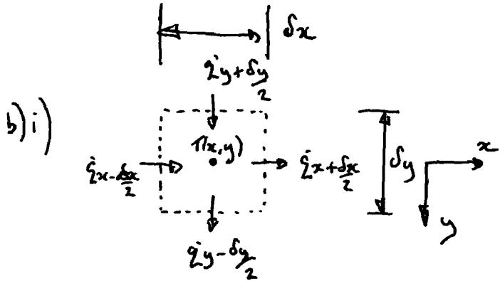
$$\text{Energy balance: } \dot{E}_{x-\frac{\delta x}{2}} - \dot{E}_{x+\frac{\delta x}{2}} + \dot{E}_{y+\frac{\delta y}{2}} - \dot{E}_{y-\frac{\delta y}{2}} = 0$$
