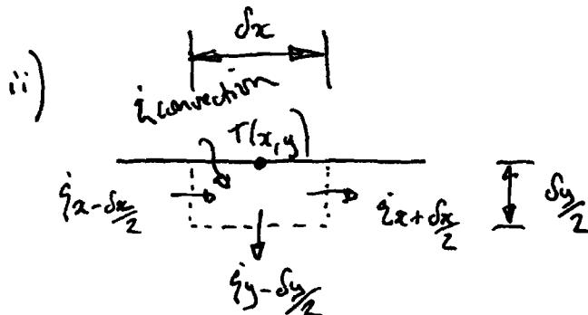
$$\text{Energy balance: } X \frac{\partial T}{\partial x} \Big|_{x-\frac{\delta x}{2}} \Big|_{y-\frac{\delta y}{2}} \left[ -X \frac{\partial T}{\partial x} \Big|_{x+\frac{\delta x}{2}} \Big|_{y-\frac{\delta y}{2}} \right] - \left( -X \frac{\partial T}{\partial y} \Big|_{y-\frac{\delta y}{2}} \Big|_{x-\frac{\delta x}{2}} \right) \frac{h \delta x (T_\infty - T_s)}{\lambda} = 0$$
