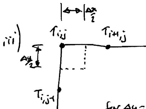
$$\Delta y \left( \frac{T_{i+1,j} - T_{i,j}}{\Delta x} \right) + \Delta x \left( \frac{T_{i,j+1} - T_{i,j}}{\Delta y} \right) + \cancel{\frac{h\alpha x}{\lambda} (T_\infty - T_{i,j}) = 0}$$
