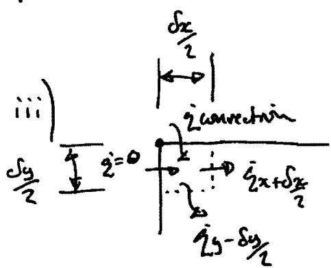
$$0 - \left( -\frac{\lambda \partial T}{\partial x} \Big|_{x+\frac{\delta x}{2}}^{\frac{\delta y}{2}} \right) - \left( -\frac{\lambda \partial T}{\partial y} \Big|_{y-\frac{\delta y}{2}}^{\frac{\delta x}{2}} \right) + \frac{h \delta x}{2} (T_\infty - T) =$$
