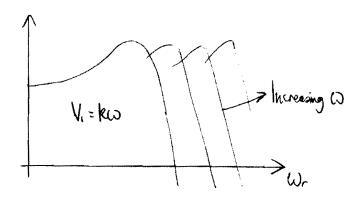
Advantages of VVVF control: the motor is always operating on the steep part of the torque-speed characteristic, so efficient; wide speed range possible at high efficiency; maximum available torque is unaffected unlike variable voltage control; motor always fully-fluxed which means it is operating efficiently and making good use of the magnetic materials.
