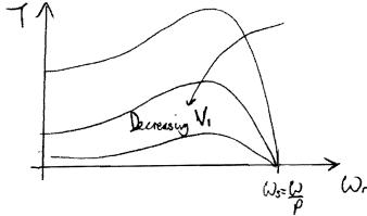
(iii) Torque-speed characteristics VVVF speed control.
