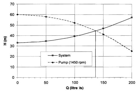
(b.ii) Transform the working conditions of the pump at 1450 rpm to the equivalent conditions at 1200 rpm. For the same pump,  $D_p$  is the same. At the equivalent running conditions, the following two parameters should be the same.
