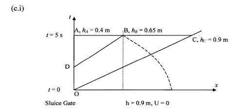
The positive characteristic OC divides the moving water and still water.
