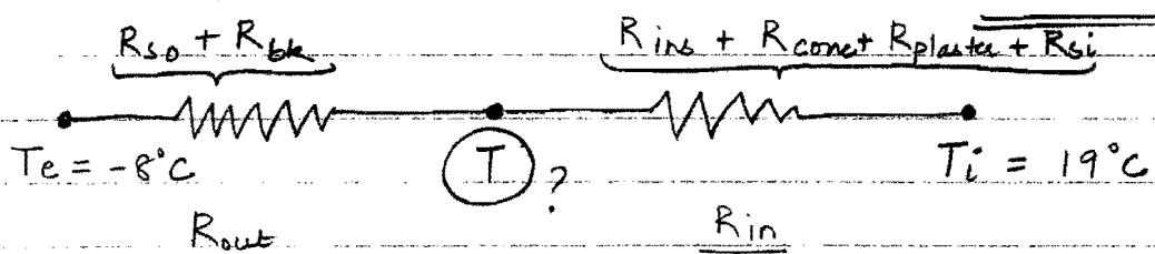
$$R_{\text{out}} = R_{\text{so}} + R_{\text{be}} = 0.16 \text{ m}^2 \text{ K/W}$$
