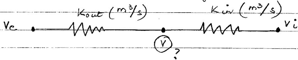
$$(\text{m}^3/\text{s}) K_{out} = \frac{A}{d_{brick}/8_{brick}} = \frac{1}{0.12/5 \times 10^{-6}} = 4.16 \times 10^{-5}$$
