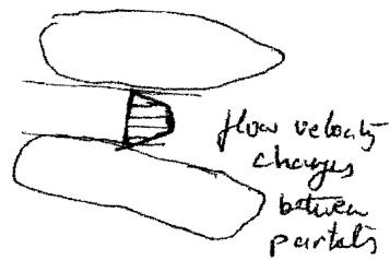
iii) Advection: Contaminant simply moves with ground water flow. This is important when ground water flow velocity is high.
