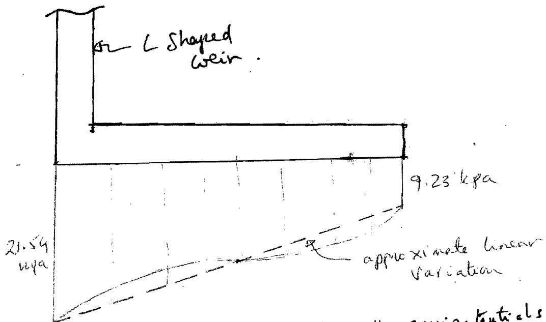
The uplift pressures can be obtained from the equipotentials on the flow net. Due to upstream blanket, the uplift pressure drops to 21.54 kPa at left edge. This drops further to 9.23 kPa on the right edge. The actual variation will be non linear due to the sloping shale bed. An approximate linear variation can be used to calculate uplift force. [10%]
