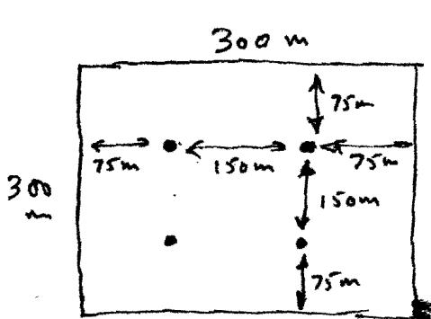
Arrange the ASTP's at 75m from edge and with 150m spacing between themselves.
