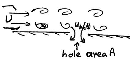
When there is a hole in the large, plane surface pressure fluctuations in the jet will drive an unsteady air flow through the hole. Denote this velocity by  $u_h(t) \propto U$
