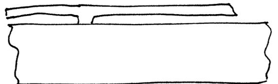
(b) MEMS acceleration sensors typically have a proof mass which flexes when the substrate suffers an acceleration, and a capacitance readout mechanism to detect the new position of the proof mass.
