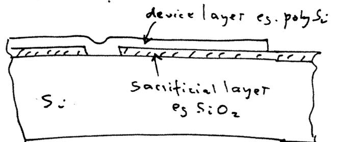
after removal of the sacrificial layer e.g. by etching in bHF the MEMS layer is suspended above the Si substrate and anchored to it where needed.
