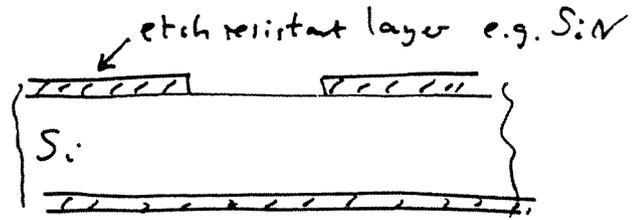
In the case of an anisotropic liquid etchant such as KOH the slow etching (111) silicon crystal planes are exposed after the etch process
