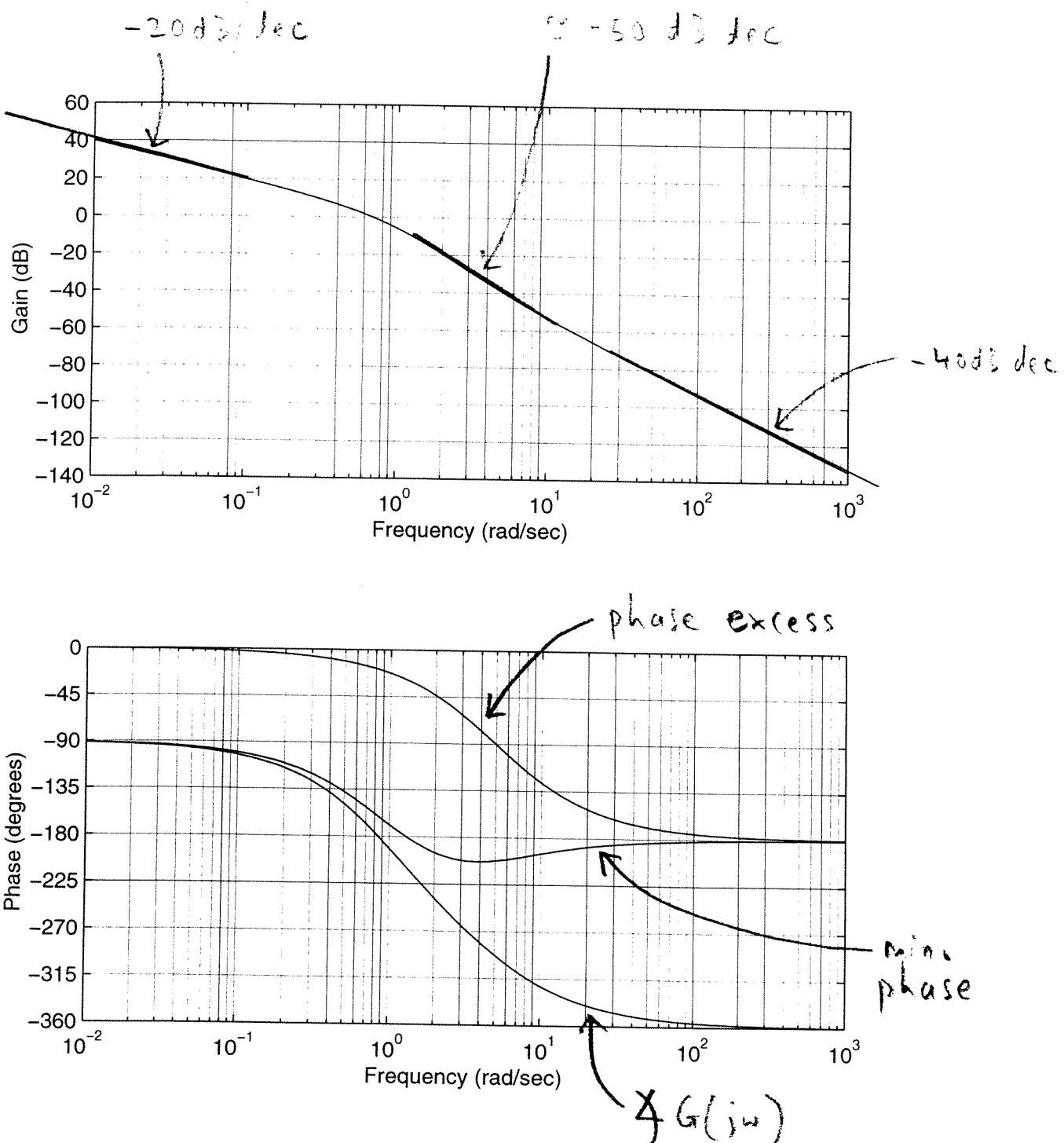
3(a) (ii) Excess phase goes from  $0^\circ$  to  $\sim 180^\circ$ . This suggests a single RHP zero at around 5 rad/sec.
