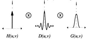
This can be a severe limitation to crosstalk in optical switches as the sidelobes are picked up by the neighbouring channels.
