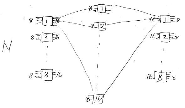
Input stage:  $\Gamma$  clossbur of dimensions  $n \times m$   $\Gamma = 8$ , n = 8, m = 16Output stage:  $\Gamma$  crossbur of clonersons  $m \times m$   $\Gamma = 8$  m = 8Centre stage: M crossbur of clonersons  $\Gamma \times \Gamma$ .
