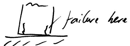
In any case a ( $\pm 65^\circ$ ) plate is not a very efficient strut.  $0^\circ$  fibres would increase the bending stiffness, but better would be to increase the second moment of area, perhaps by using a tube or square section, or a sandwich panel construction. Again end fittings will be needed.
